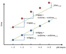
Fig. 5. Jitter calculation
