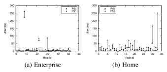
Fig. 6. The  $50^{th}$  and  $95^{th}$  percentile of jitter distribution across hosts. Jitter variation is much higher in residential networks than in enterprise networks. Figure 6(b) shows that  $95^{th}$  percentile jitter values is significantly worse than the median jitter values in home networks.
