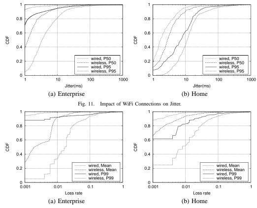
Fig. 12. Impact of WiFi Connections on Packet Loss.
