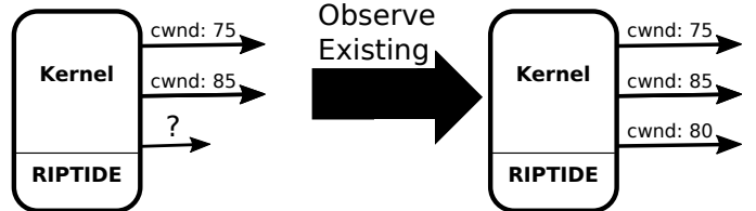
Fig. 7: The core principle of Riptide is to set new initcwnds according to observed behavior.
